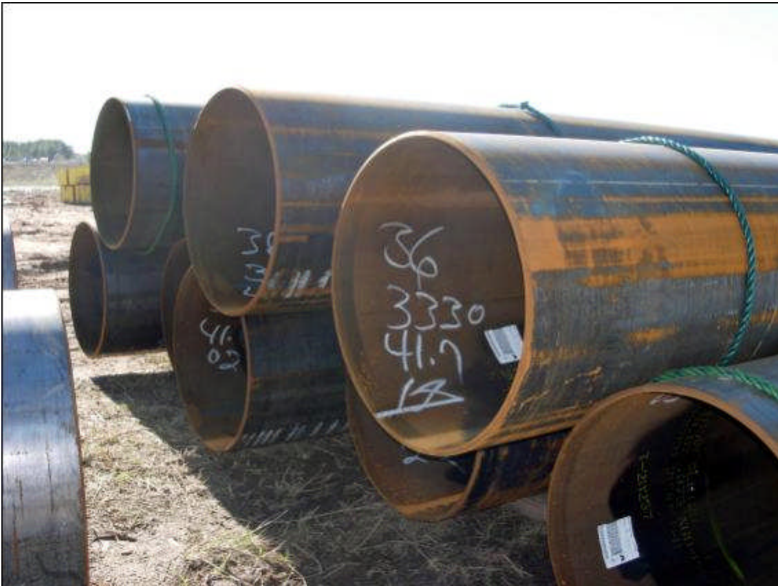
Figure 29. Line pipe. Courtesy Pipeline Knowledge & Development.
