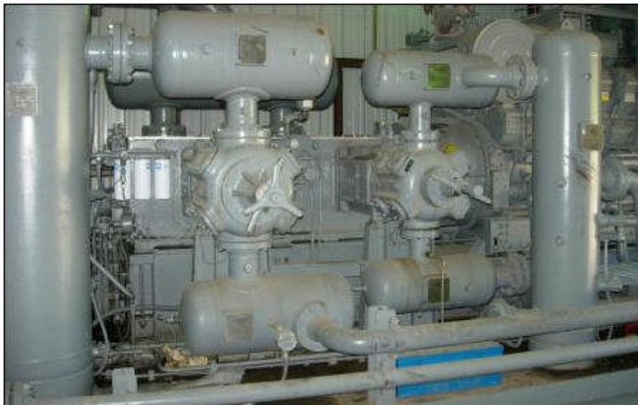
Figure 16. Reciprocating compressor connected to an engine with a shaft. Courtesy Pipeline Knowledge & Development.
